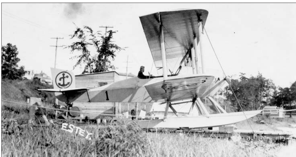
Side view of the seaplane; in a 1916 letter, Estey wrote, "It is made of steel throughout and ...a special linen covered with a fire and waterproof coating, which forms the wings, tail and rudder. It carries two machine guns, a pilot, observer and gunner; also 50 gallons of gasoline. It is 48 feet from tip to tip of wings with an 8 foot depth, weighs 2000 pounds and is equipped with a 140 hp Sturtevant motor which will drive this big machine 105 mph." Note the Rhode Island insignia on the tail and bottom of wings.
